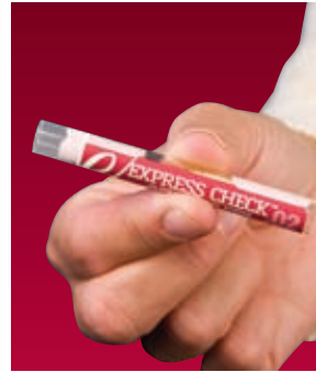
To perform test, the user first crushes the test between fingers.
